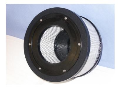
Size: Connection: Weight: 224mm OD x 169mm ID x 180mm long 6 off M5 nut certs equi-spaced on 197 PCD 1.37Kg
